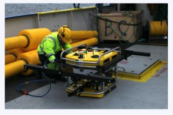
The MX3D UW is an **open system**. Being located on the ROV/ROTV, the MX3D UW electronics transmits the data via TCP/IP to the vessel, thus allowing for a highly flexible integration of the MX3D UW in existing systems.
